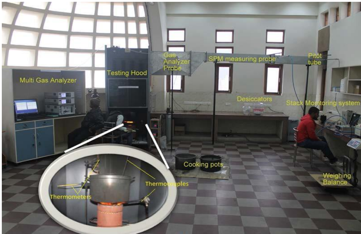
fig.5. Biomass cookstove testing & certification centre at SSS-NIBE
